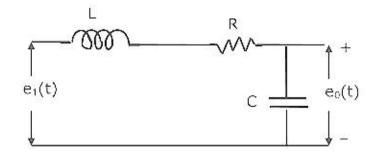
2.6. A series R-L-C circuit has the following parameter values: R  $10\Omega$ , L = 0.01 H, C = 100 mF.
