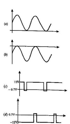
20. A single-phase half wave uncontrolled converter circuit is shown in figure. A 2-winding transformer is used at the input for isolation. Assuming the load current to be constant and v = V<sub>m</sub> sin ωt, the current waveform through diode D<sub>2</sub> will be
