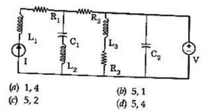
30. The parameter type and the matrix representation of the relevant two port parameters that describe the circuit shown are
