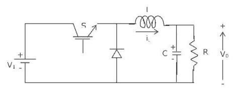
duty ratio D. what is the value of D at the boundary of continual discontinuous conduction of the inductor current i<sub>1</sub>?
