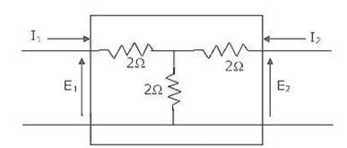
The admittance parameters  $Y_{11}$ ,  $Y_{12}$ ,  $Y_{22}$  for the network shown are
