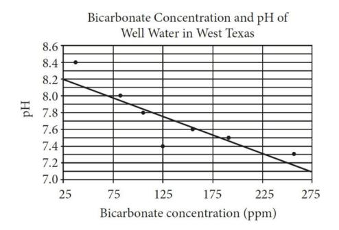
The scatterplot above shows the pH of seven well water samples in West Texas with respect to the bicarbonate concentration in ppm (parts per million). The line of best fit is also shown.
