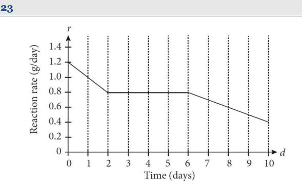
The graph above represents the reaction rate, r, at which an unfinished iron nail rusts in water during the first 10 days of an
