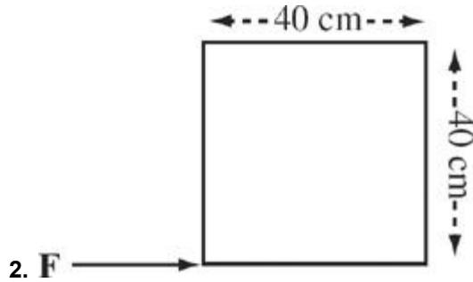
The figure above shows a square metal plate of side length 40 cm and uniform density, lying flat on a table. A force  $F$  of magnitude 10 N is applied at one of the corners, parallel to one of the sides, as shown. What's the torque produced by  $F$  relative to the center of the square?
