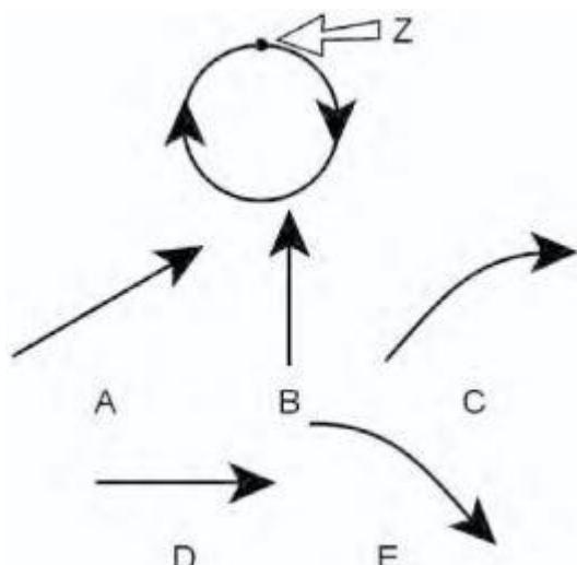
13. An object on a string is traveling in a circular path as shown. If the string breaks when the object is at point Z, which pathway will the object follow?
