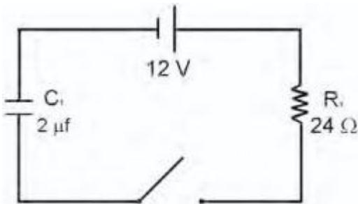
7.  $C_1$  is an uncharged capacitor (shown in the circuit above). At  $t = 0$  the switch (SW1) is closed, and  $C_1$  begins to charge.
