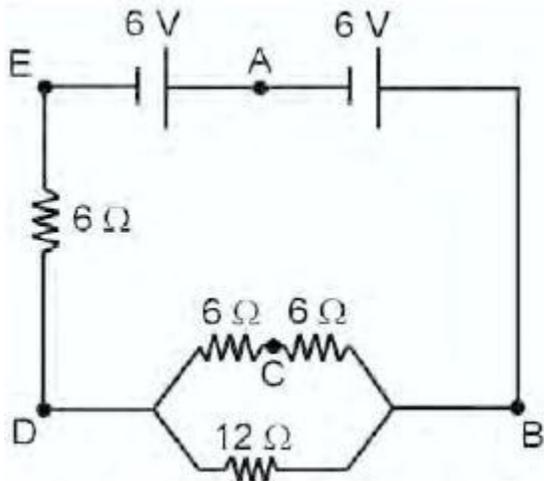
At which point is all the voltage in the circuit dropped to zero?
