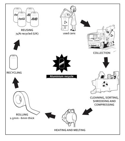
The diagram illustrates how aluminium cans are recycled. First, the cans need to be taken to special collection centres instead of being thrown away with the normal refuse. The cans are collected from here and taken to a factory where they are first sorted and then cleaned. Next, the cans are shredded and crushed in a special machine.
