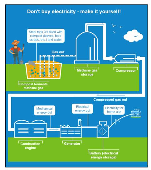
The diagram shows a process for producing electricity for home use. The equipment consists of a large tank, boxes and pipes that would be able to fit into a garage-sized room.
