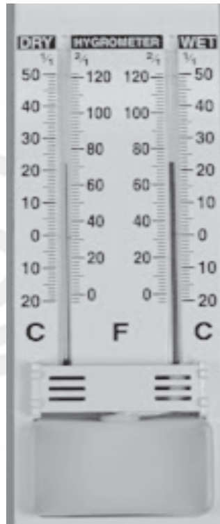
Fig. 2.3: Wet and dry bulb hygrometer (Psychrometer).
