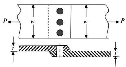
plate width w = 200 mmplate thickness t = 5 mmnumber of rivets n = 3rivet diameter  $d_r = 10 \text{ mm}$ rivet hole diameter  $d_h = 11 \text{ mm}$ allowable tensile stress of plate  $\sigma_p = 200 \text{ MPa}$ allowable bearing stress of rivet  $\sigma_c = 150 \text{ MPa}$
