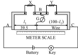
In a meter bridge, as shown in the figure, it is given that resistance  $Y = 12.5 \Omega$  and that the balance is obtained at a distance 39.5 cm from end A (by Jockey J). After interchanging the resistances X and Y, a new balance point is found at a distance  $l_2$  from end A. What are the values of X and  $l_2$ ? (1) 19.15  $\Omega$  and 60.5 cm (2) 8.16  $\Omega$  and 60.5 cm (3) 8.16  $\Omega$  and 39.5 cm (4) 19.15  $\Omega$  and 39.5 cm **Ans.** (2)
