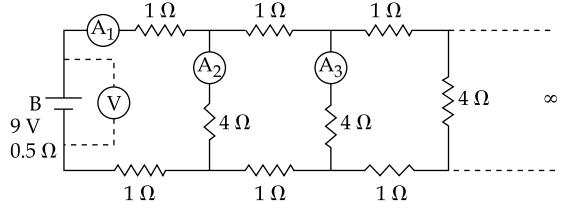
A 9 V battery with internal resistance of  $0.5 \Omega$  is connected across an infinite network as shown in the figure. All ammeters  $A_1$ ,  $A_2$ ,  $A_3$  and voltmeter  $V$  are ideal.
