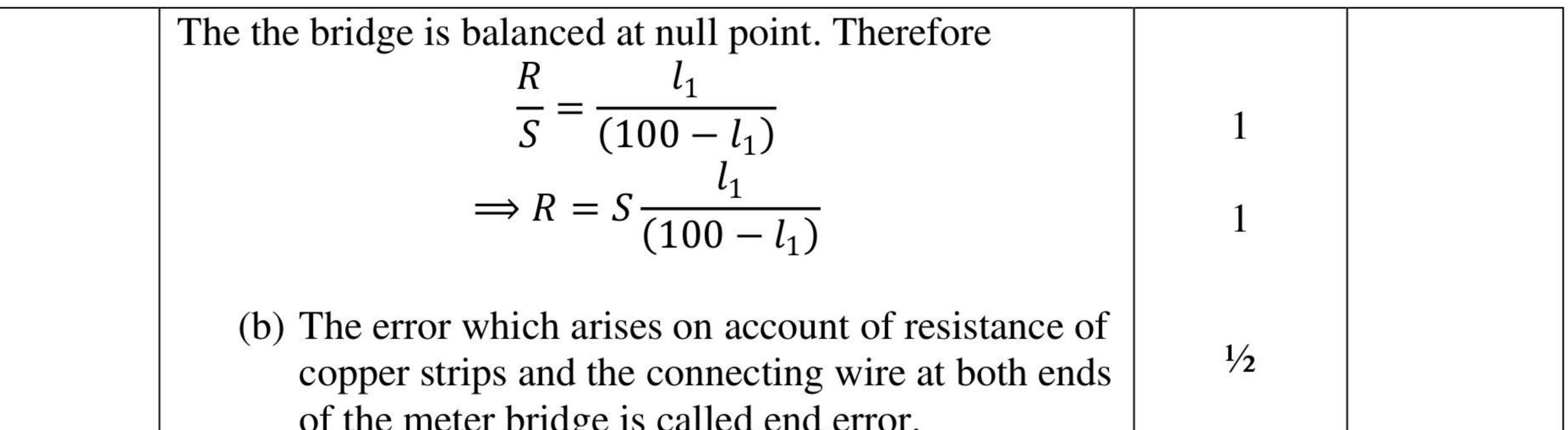
of the meter bridge is called end error. It is minimized by adjusting the balance point near the middle point of the bridge. No effect, as the bridge remains balanced. OR (a) Statement of working Principle Circuit diagram and determination of internal resistance (b) (i) Effect of internal resistance Review Platform 1/2(ii) Series resistance
