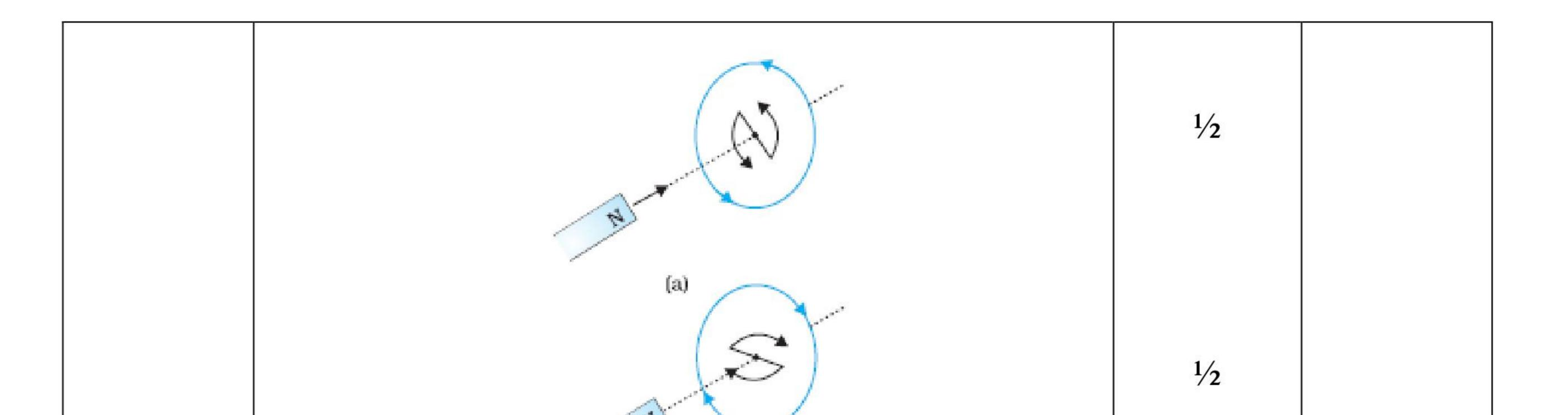
When the north pole of a bar magnet is pushed towards the close coil, the magnetic flux through coil increases and the current is induced in the coil in such a direction that it opposes the increase in flux. This is possible when Jeview Platform the induced current in the coil is in the anticlockwise direction. Just the opposite happens when the north pole is moved away from the coil. In either case, it is the work done against the force of
