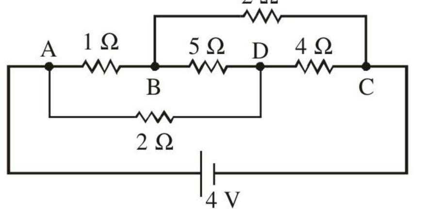
Calculate the current drawn from the battery by the network of resistors shown in the figure.
