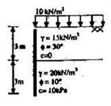
CE.13.A group of 16 piles (diameter = 50 cm, length = 14m, centre to centre spacing = 1m) arrange in a square pattern passes through a recent fill (thickness = 3 m) overlying a soft clay deposit (thickness = 5m) which is consolidating under the fill load and rests in a stiff clay strata. All the strata are saturated. The soil properties of different strata are
