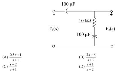
Q.5 Assuming zero initial condition, the response y(t) of the system given below to a unit step input u(t) is
