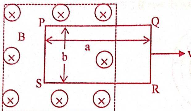
As shown in figure, a rectangular loop of length 'a' and width 'b' and made of a conducting material of uniform cross-section is kept in a horizontal plane where a uniform magnetic field of intensity  $B$  is acting vertically downward. Resistance per unit length of the loop is  $\lambda \Omega/m$ . If the loop is pulled with uniform velocity 'v' in horizontal direction, which of the following statement is/are true ?
