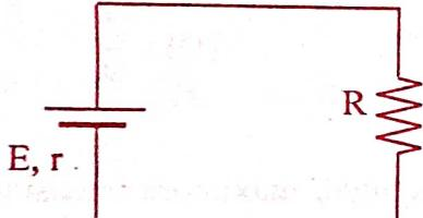
A battery of emf  $E$  and internal resistance  $r$  is connected with an external resistance  $R$  as shown in the figure. The battery will act as a constant voltage source if
