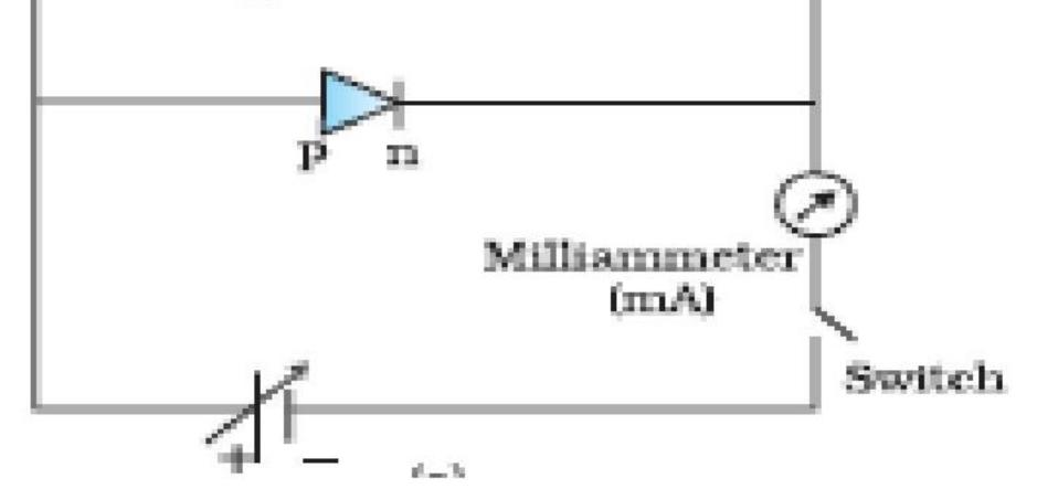
In the forward bias the width of depletion layer decreases and barrier height is reduced.
