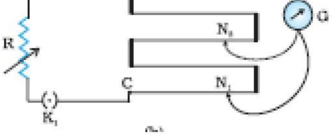
The cell (emf E) whose internal resistance is to be determined is connected across a resistance box through a key  $K_2$ , as shown in figure above. With key  $k_2$  open. Balance point is obtained at length  $l_1(AN_1)$ Then,
