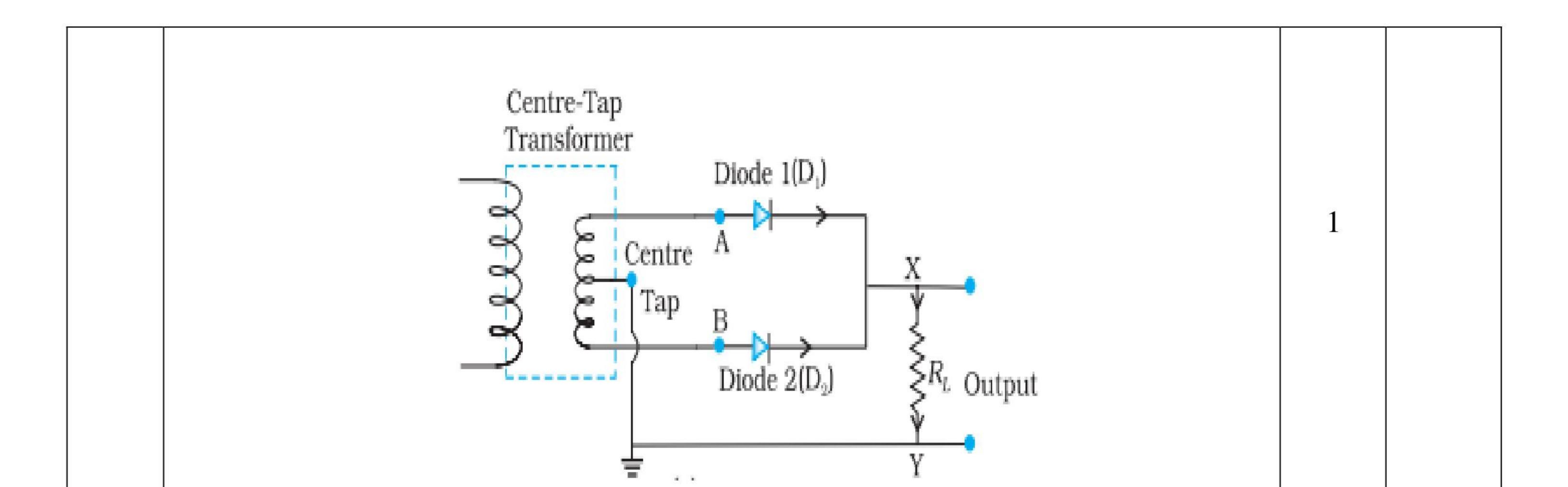
Working: The input voltage to A with respect to the centre tap at any instant is positive, At that instant voltage at B being out of phase will be negative. So diode D<sub>1</sub> gets forward biased and conducts while D<sub>2</sub> being reversed biased and does not conduct. Hence during this positive half cycle, we get an output current.
