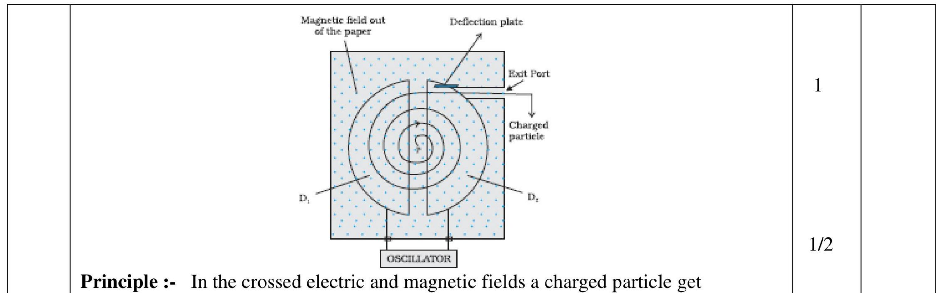
accelerated and its frequency of revolution in the magnetic field is independent of its energy.
