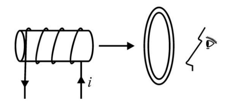
Figure shows a current carrying solenoid moving towards a conducting loop. Find the direction of the current induced in the loop.
