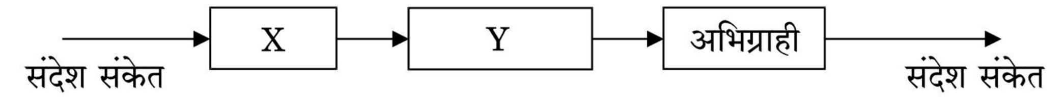
Name the boxes X and Y shown in the block diagram of a generalized communication system:
