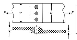
plate width w = 200 mmplate thickness t = 5 mmnumber of rivets n = 3rivet diameter  $d_r = 10 \ mm$ rivet hole diameter  $d_h = 11 \ mm$ allowable tensile stress of plate  $\sigma_p = 200 \text{ MPa}$ allowable bearing stress of rivet  $\sigma_c = 150 MPa$
