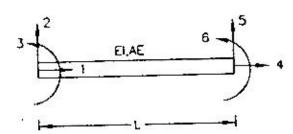
$$K = \frac{EL}{L^3} \begin{bmatrix} \frac{AL^2}{I} & \text{Symmetric} \\ 0 & 12 \\ 0 & 6L & 4L^2 \\ -\frac{AL^2}{I} 0 & 0 & \frac{AL^2}{I} \\ 0 & -12 & -6L & 0 & 12 \\ 0 & 6L - 2L^2 & 0 & -6L & 4L^2 \end{bmatrix}$$
