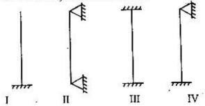
It is required to order these four beams in the increasing order of their respective first buckling loads. The correct order is given by
