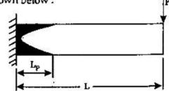
The length L, of the plastic zone, when the maximum bending moment, equals the plastic moment M<sub>p</sub>, given by
