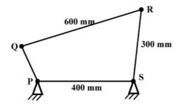
For the mechanism to be a crank-rocker mechanism, the length of the link PQ
