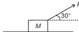
If  $M = 10 \text{ kg}$  and coefficient of friction is  $0.25$ , find minimum  $F$  so that block slides
