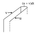
Consider area A of the plate moving towards right (see figure). In next dt time, only those particles of the gas can collide with the plate (on its right face) as are within (v + u) dt distance from it. Number of these particles = n(u + v) dt A, where n is number of gas particles per unit volume. Only half of these particles will collide with the plate, the other half will be moving away from it.
