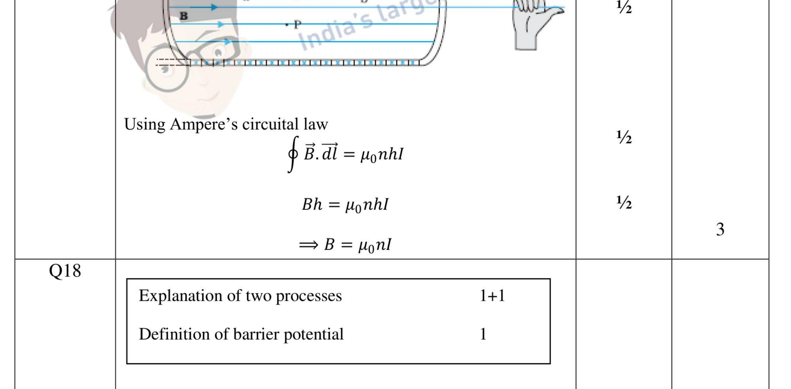
Diffusion: It is the process of movement of majority charge carriers from their majority zone (.i.e., electrons from  $n \rightarrow p$  and holes from  $p \rightarrow n$ ) to the minority zone across the junction on account of different concentration
