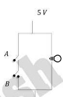
When both A and B are open or any one of them is open, bulb will glow. When both switches are closed, due to short circuit, bulb will not glow.
