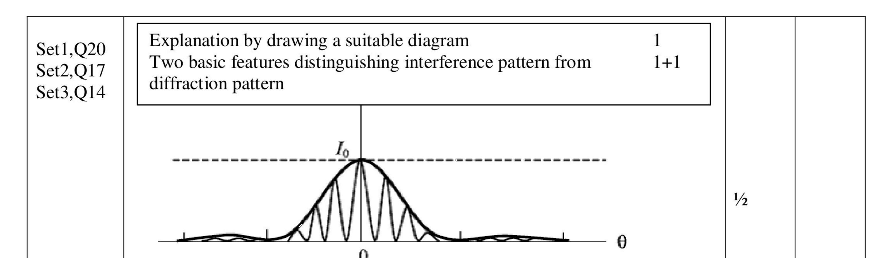
The diagram, given here, shows several fringes, due to double slit interference, 'contained' in a broad diffraction peak. When the seperation between the slits is large compared to their width, the diffraction pattern becomes very flat and we observe the two slit interference pattern. [Note: The students may be awarded 1 mark even if they just draw the diagram.]
