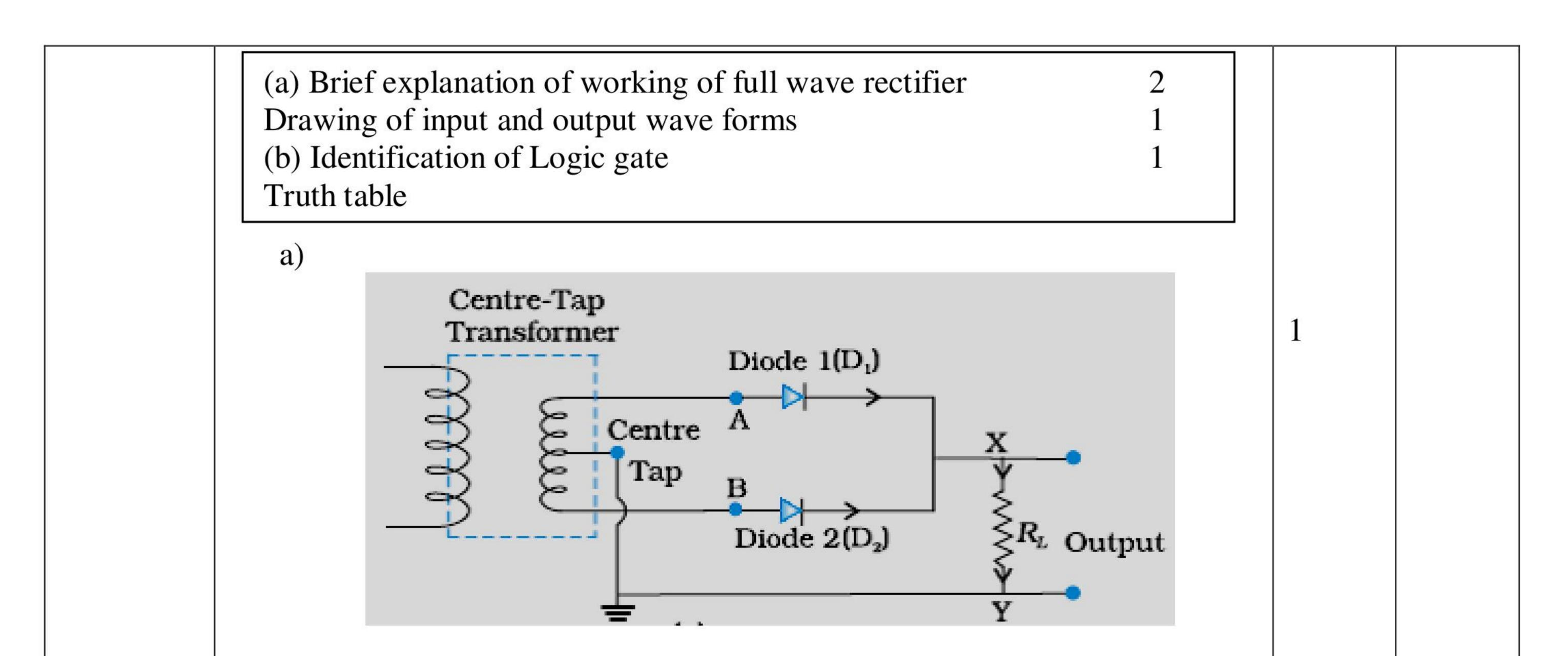
For half cycle of input ac, one diode out of the two, will get forward biased and will conduct, while the other diode, being reverse biased, will not conduct. For other cycle of input signal, the diode, which was reverse biased, will get forward biased and will conduct, and the other diode will get reverse biased and will stop conducting. Hence we obtain a unidirectional output voltage for the positive as well as for negative half cycles.
