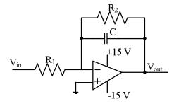
(A) low pass filter.(C) high pass filter.
