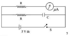
Two resistances of same value, one capacitor and one micro ammeter is connected to a 5V battery of negligible internal resistance and a switch (s) as shown in the figure. When the switch is closed the micro ammeter shows a reading of 20  $\mu$ A.
