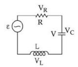
If 'q' is the charge on the capacitor and 'i' is the current, from Kirchoff's loop rule :
