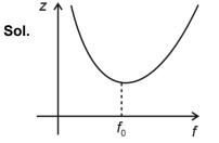
⇒ When frequency of the ac source is increased from  $f_0$  to  $2f_0$  then impedance of the circuit increases.
