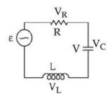
If 'q' is the charge on the capacitor and 'i' is the current, from Kirchoff's loop rule :
