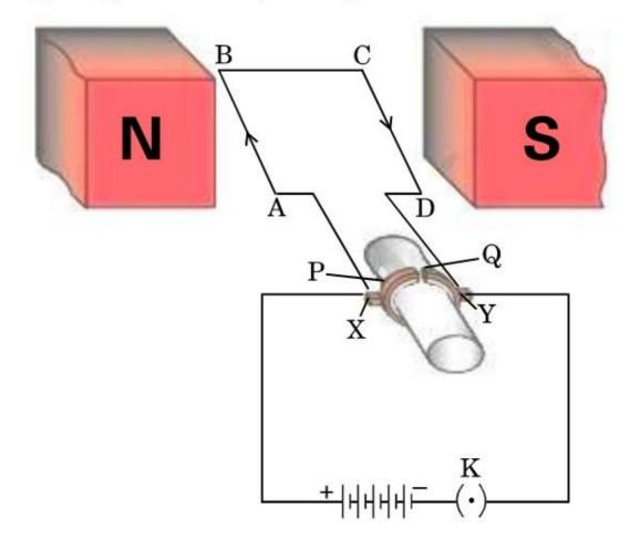
(b) In the figure given below, a simple electric motor is shown :
