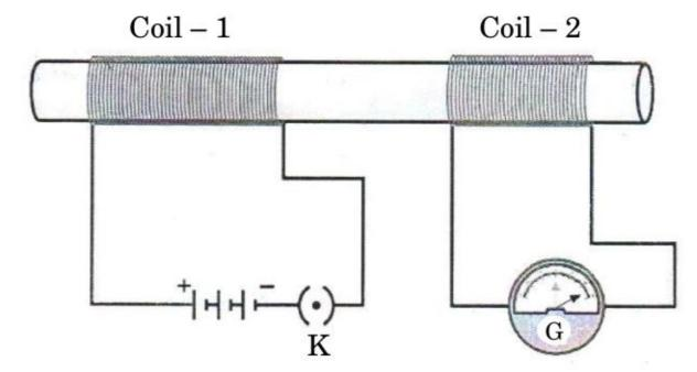
(i) Why does the galvanometer show deflection only when the key (K) is plugged in and not when a steady current starts flowing in the circuit?
