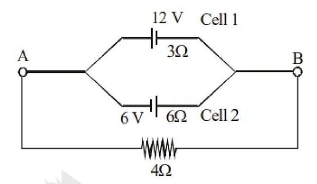
$$egin{aligned} E_{eq} &= rac{rac{12}{3} - rac{6}{6}}{rac{1}{3} + rac{1}{6}} \ E_{eq} &= 6 V \ r_{eq} &= 2 \Omega \ R &= 4 \Omega \end{aligned}$$
