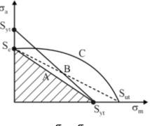
Line A represents Soderberg line,  $\frac{\sigma_a}{S_e} + \frac{\sigma_m}{S_{vt}} = 1$
