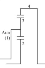
m = 8 mm T<sub>2</sub> = 19, T<sub>3</sub> = 24, N<sub>2</sub> = 0, N<sub>4</sub> = 20 rpm CCW r<sub>4</sub> = r<sub>2</sub> + 2r<sub>3</sub>  $m\frac{T_4}{2} = \frac{mT_2}{2} + 2 \times \frac{mT_3}{2}$ T<sub>4</sub> = T<sub>2</sub> + 2T<sub>3</sub> = 19 + 2 × 24 = 67 By relative velocity method  $\frac{N_2 - N_a}{N_4 - N_a} = \left(-\frac{T_3}{T_2}\right) \times \left(\frac{T_4}{T_3}\right) = -\frac{T_4}{T_2}$ {Considering CCW as +ve}  $\frac{0 - N_a}{20 - N_a} = -\frac{67}{19} = -3.526$
