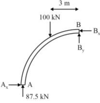
$\Sigma M_B = 0$   $A_x \times 6 = 87.5 \times 6 - 100 \times 3$   $A_x = 37.5 \text{ kN}$   $\Sigma F_x = 0$  $B_x = A_x = 37.5 \text{ kN}$
