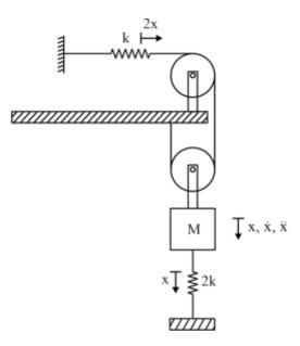
For excessively large oscillation of mass M, the driving frequency ( $\omega$ ) should be equal to natural undamped frequency ( $\omega_n$ ).
