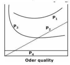
A. Curve P<sub>1</sub> total cost, P<sub>2</sub> Holding cost, P<sub>3</sub>: setup cost, P<sub>4</sub>: production cost
