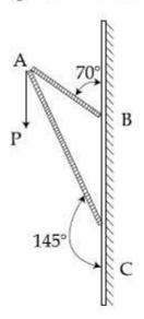
Suppose the force is  $\overrightarrow{P}$  resolved parallel to the arms AB and AC of the frame.
