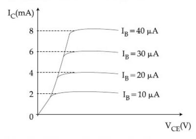
The estimated current gain from the figure is \_\_\_\_\_
