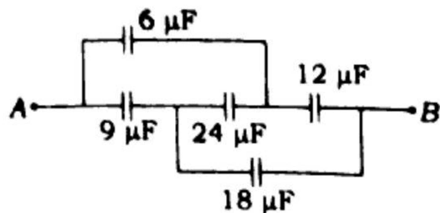
With reference to the combination of capacitors shown the equivalent capacitance  $C_{AB}$  between the points A and B is
