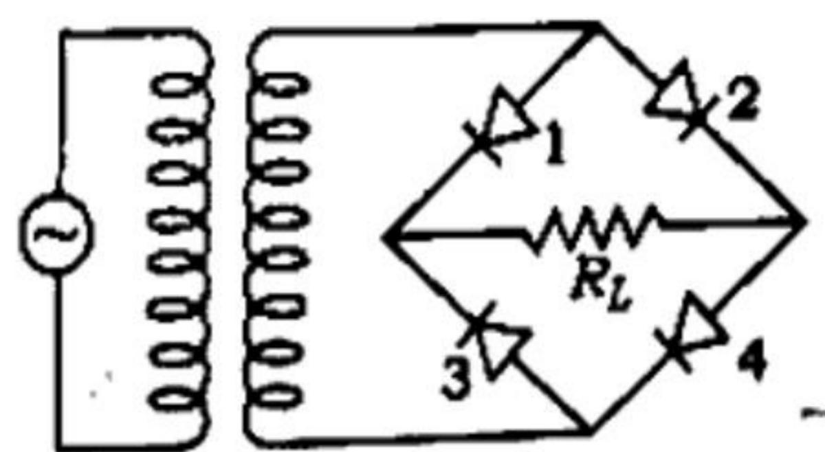
Detect the diode connection which is faulty?
