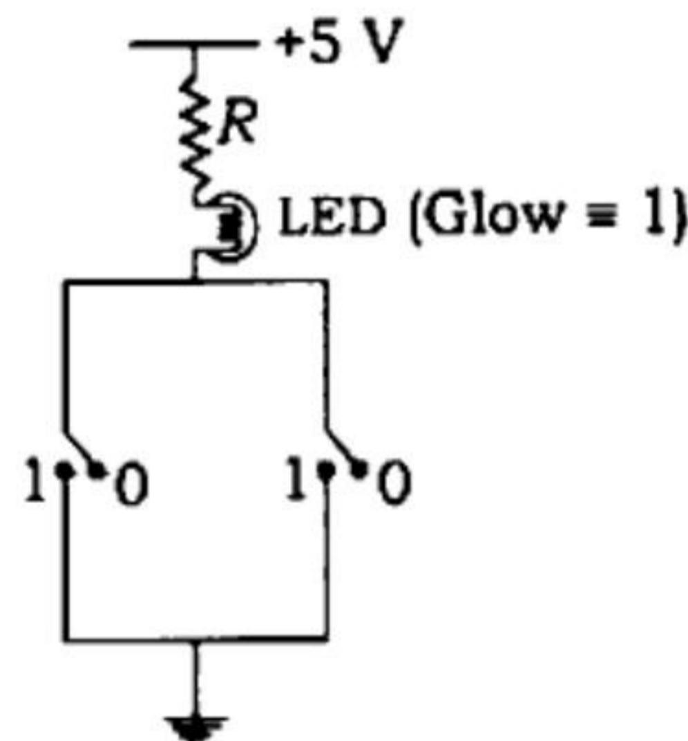
The equivalent logic gate represented by the circuit above is
