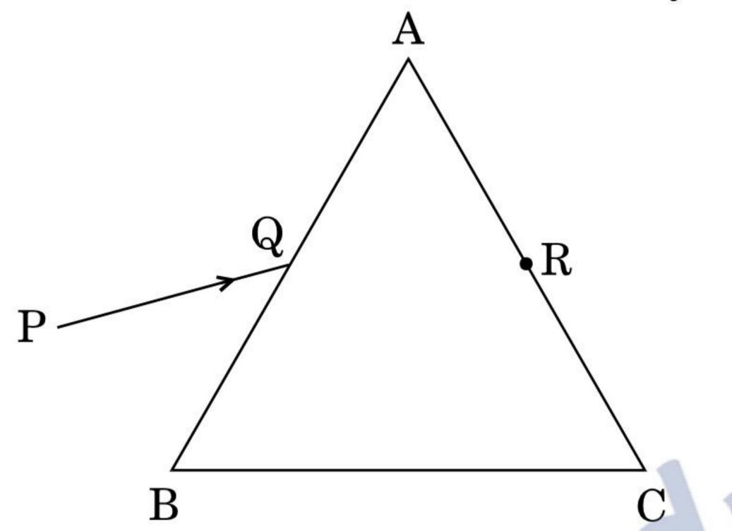
Draw the ray diagram showing the passage of the ray through the prism. If the angle of the prism is  $60^\circ$  and refractive index of the material of the prism is  $\sqrt{3}$ , determine the values of angle of incidence and angle of deviation.
