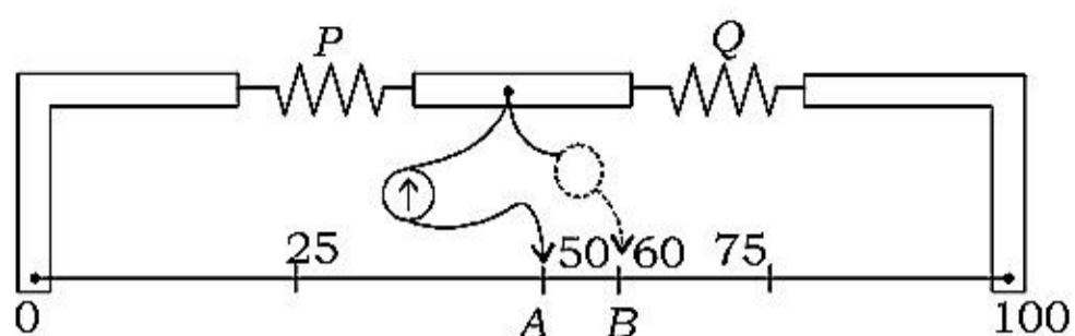
When two equal unknown resistances  $Y$ , each are inserted in the gaps  $P$  and  $Q$  of the meter bridge as shown, the null appears at the middle  $A$ . But if a  $10\ \Omega$  resistance is connected parallel to  $Y$  at  $Q$ , the null shifts  $10\text{ cm}$  to the right at  $B$  as shown. The value of  $Y$  is
