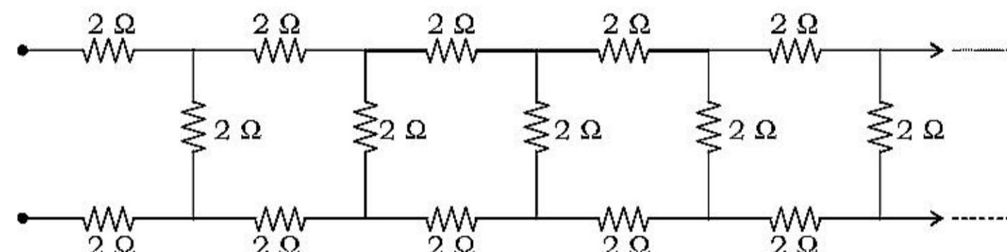
The nearest value of equivalent resistance of the combination of resistances given above is
