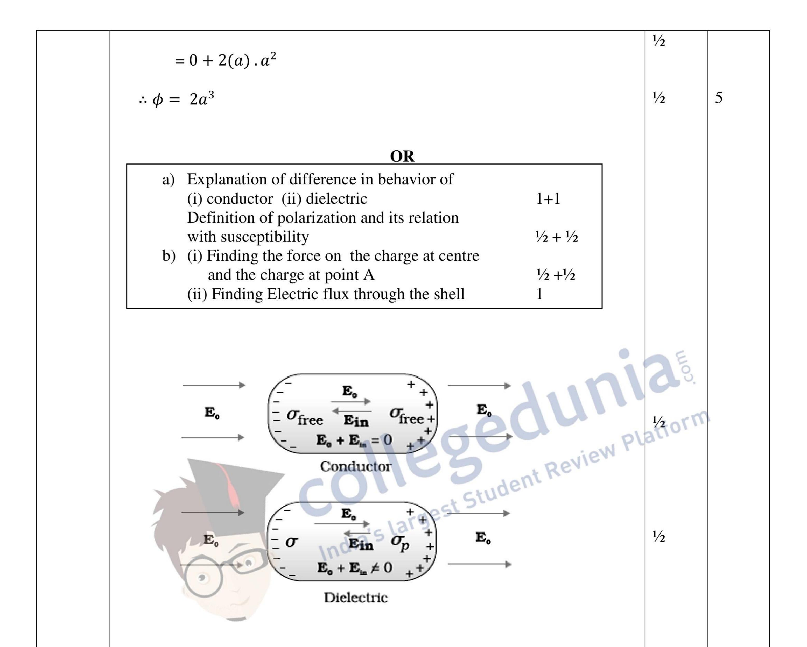
In the presence of Electric field, the free charge carriers, in a conductor, move the charge distribution in the conductor readjusts itself so that the net Electric field within the conductor becomes zero.
