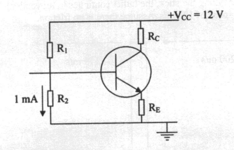
Given that  $V_E = 2 \text{ V}$ ,  $V_{BE} = 0.6 \text{ V}$  and  $I_C \cong I_E$ , find the values needed for the resistances  $R_1$ ,  $R_2$ ,  $R_E$  and  $R_C$ . (15)
