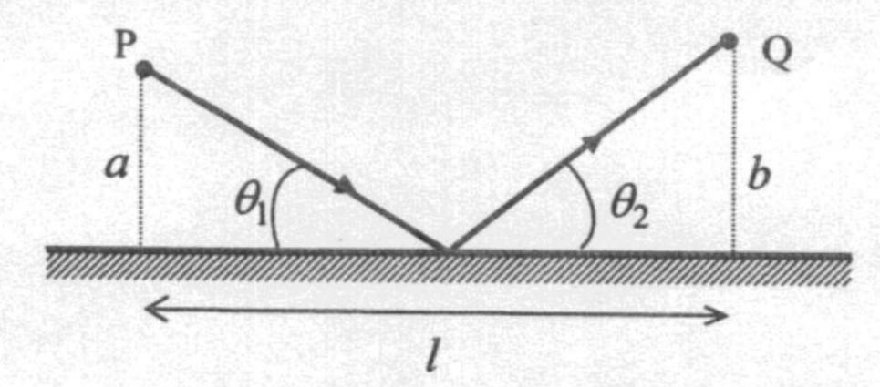
Show that the incident and reflected light make the same angle from the mirror using Fermat's principle (light travels from P to Q by taking a path such that the time of travel is the least).
