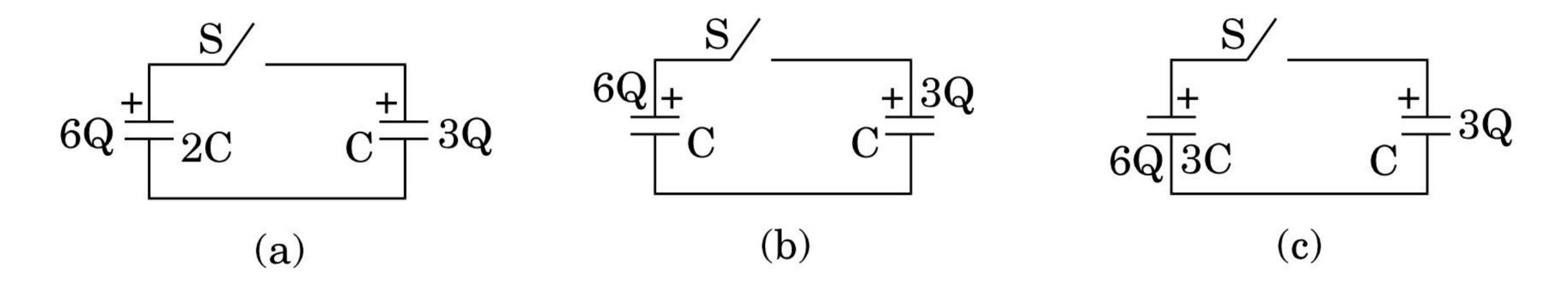
Three circuits, each consisting of a switch 'S' and two capacitors, are initially charged, as shown in the figure. After the switch has been closed, circuit will the charge on the left-hand which capacitor ın (i) increase, (ii) decrease and (iii) remain same? Give reasons.
