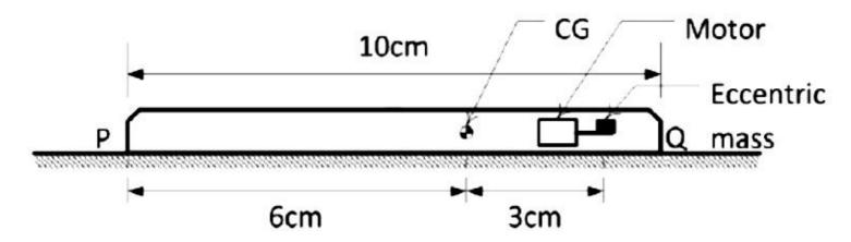
Given in addition that the eccentric mass = 2 grams, eccentricity = 2.19 mm, mass of the mobile = 90 grams,  $g = 9.81 \text{ m/s}^2$ . Uniform speed of the motor in RPM for which the mobile will get just lifted off the ground at the end Q is approximately
