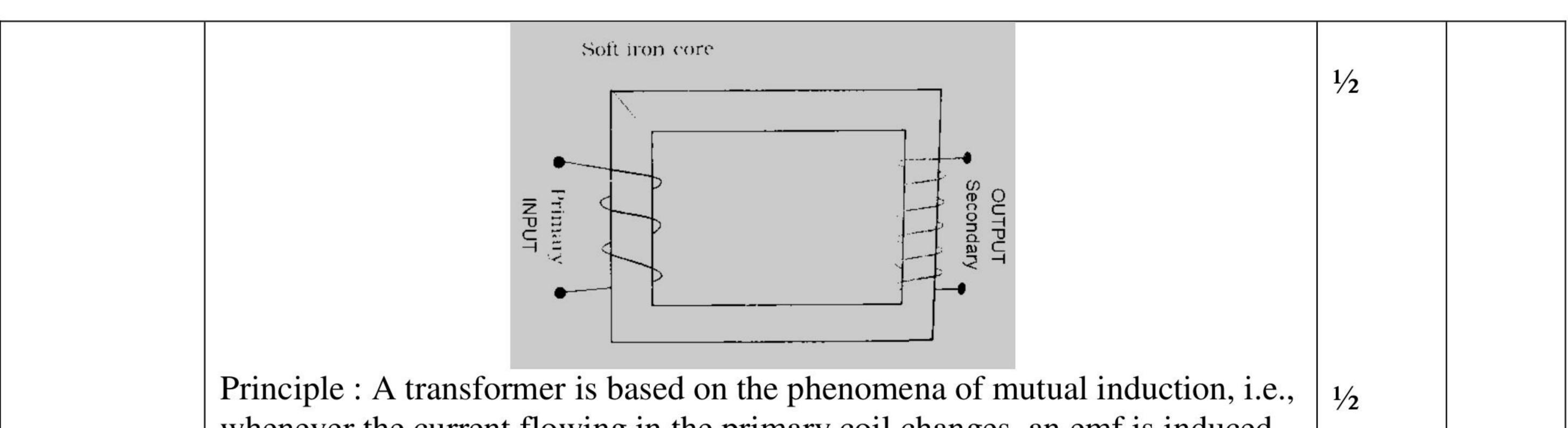
whenever the current flowing in the primary coil changes, an emf is induced in the secondary coil.
