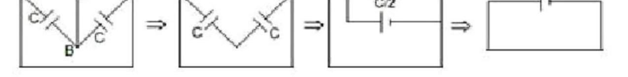
Here  $V_A = V_B$  (A & B are at the same potential) so the bridge capacitor can be removed.
