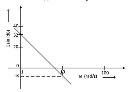
The gain  $(20 \log |G(s)|)$  is 32 dB and -8 dB at 1 rad/s and 10 rad/s respectively. The phase is negative for all  $\omega$ . Then G(s) is
