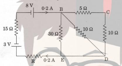
Calculate the value of the resistance R in the circuit shown in the figure so that the current in the circuit is 0.2 A. What would be the potential difference between points B and E?
