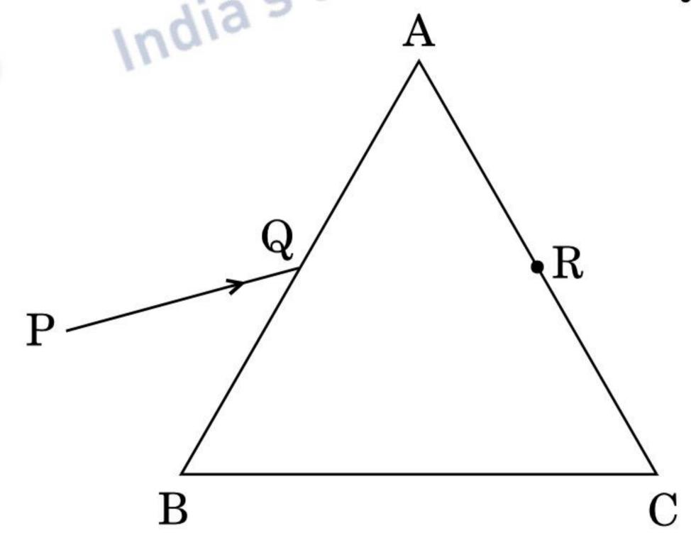
Draw the ray diagram showing the passage of the ray through the prism. If the angle of the prism is  $60^{\circ}$  and refractive index of the material of the prism is  $\sqrt{3}$ , determine the values of angle of incidence and angle of deviation.
