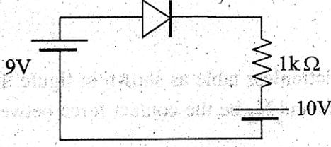
What is the value of current through the diode in the circuit given ?
