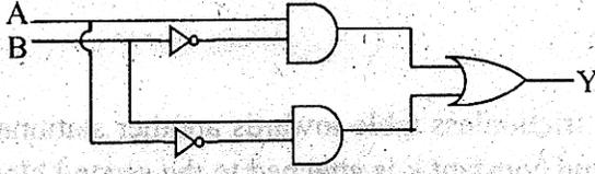
For the given logic circuit, the output Y for inputs  $(A = 0, B = 1)$  and  $(A = 0, B = 0)$  respectively are
